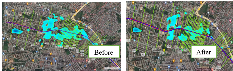
Figure 10. Before and after drainage modification for Jalan Pontian-Batu Pahat catchment.
