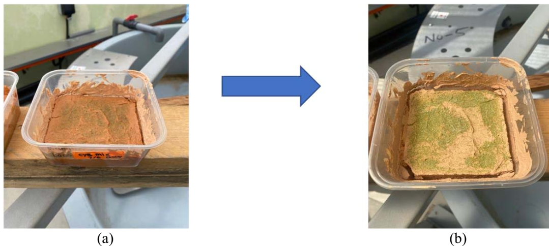
Figure 5. The visual appearance of the growth of C3 strain on soil sample at a) day 0 and b) day 7
