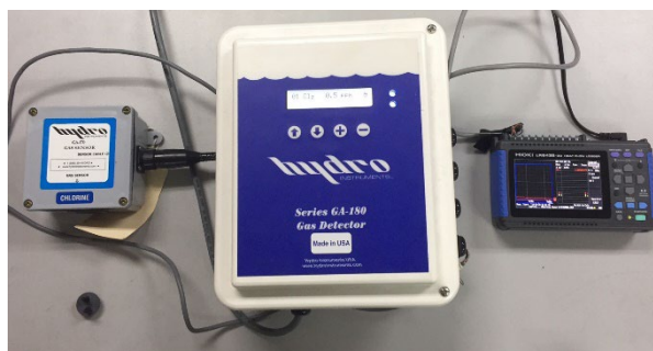
Figure 2. HYDRO chlorine gas detector and Data Logger HIOKI-LR 8431-20.
