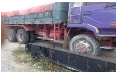
Figure 14a. 24 tonnes truck with a full load of sand material in the OMA test at the weighing station for the weight measurement of the front axle.
