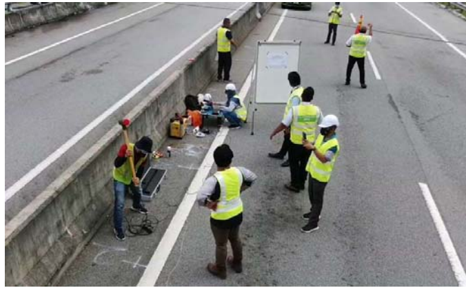
Figure 9. Stage of loading by hammering the deck to generate the responses
