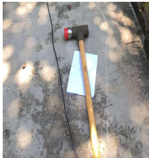
Figure 10b. Modal hammer (model TLD086D50).
