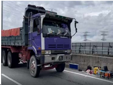
Figure 13a. 24 tonnes truck with a full load of sand material moving along the 32 m path length for the OMA test.
