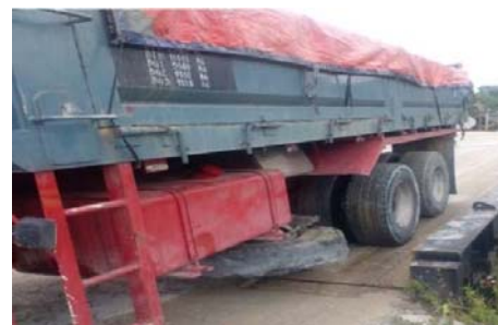
Figure 14b. 24 tonnes truck with a full load of sand material loaded used for the OMA test at the weighing station for the weight measurement of the rear axle.
