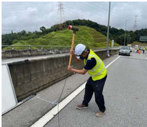
Figure 6a. A hitting point in progress to get bridge response in the form of frequency and mode shapes.
