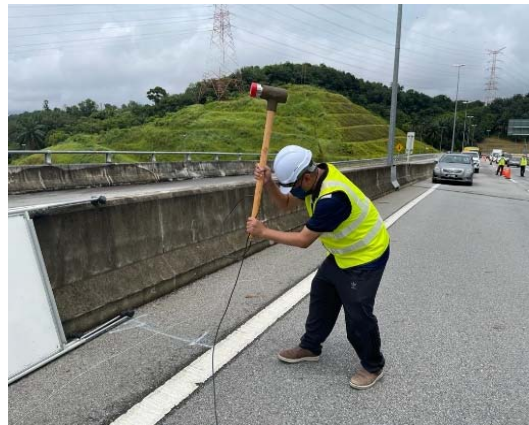
Figure 20b. Hammering of excitation points for the modal test (also known as Experimental Modal Analysis-EMA).
