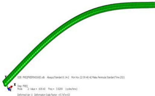
Figure 22a. First Bending Mode shape (3.929 Hz) based on numerical analysis (Abaqus).
