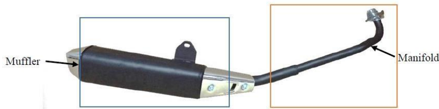
Figure 1. Components of an exhaust system
