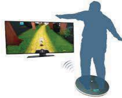
Figure 2. Game-based software modules with instant visual feedback provided by the FIBOD wobble board.
