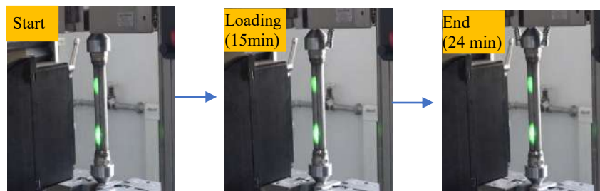
Figure 7. Tensile deformation morphology at loading time of 24min
