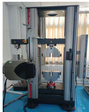
Figure 5. Z250SNS electronic universal testing machine
