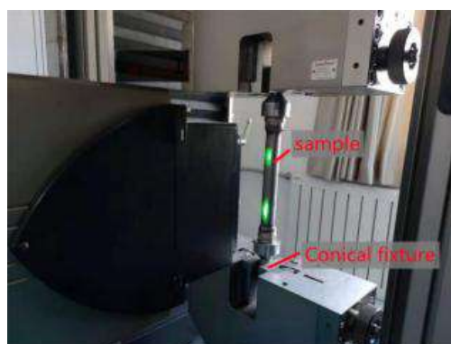
Figure 6. Tensile test clamping
