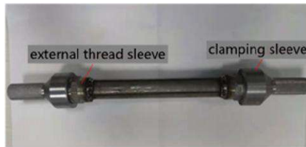
Figure 4. Tensile clamping device for O-core metal sandwich structure pipe
