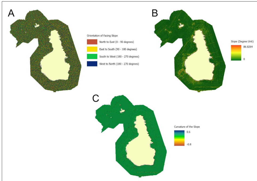
Figure 5. Bathymetric derivatives derived from bathymetric map. (a) aspect, (b) slope, and (c) curvature.
