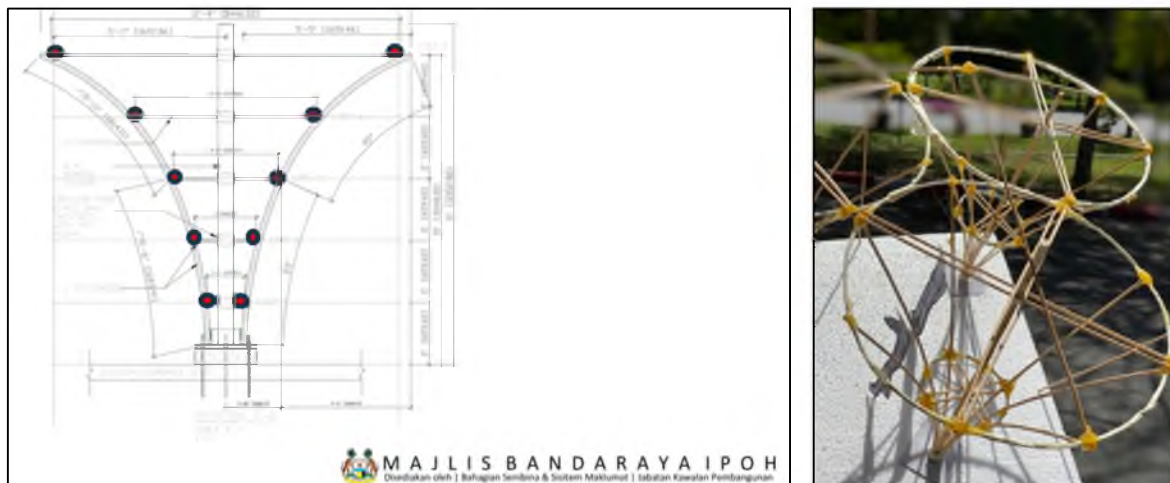
Figure 5. Section and Model of Bamboo Pavilion, red color indicates proposed rings (Pilot Test Model) and a central post from Buloh Betong.
