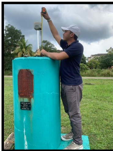
Figure 4. GNSS equipment mounted on pillar
