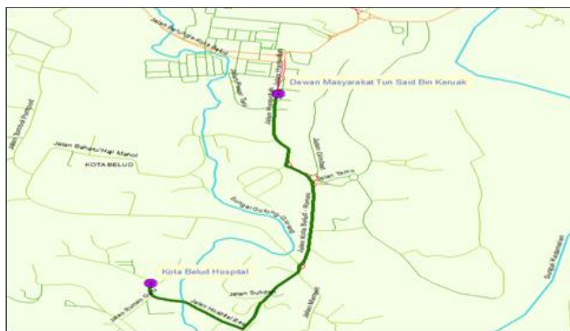
Figure 6. Normal route design using ArcGIS network analyst from Kota Belud hospital to Dewan Masyarakat (community hall) Tun Said Keruak (temporary shelter)
