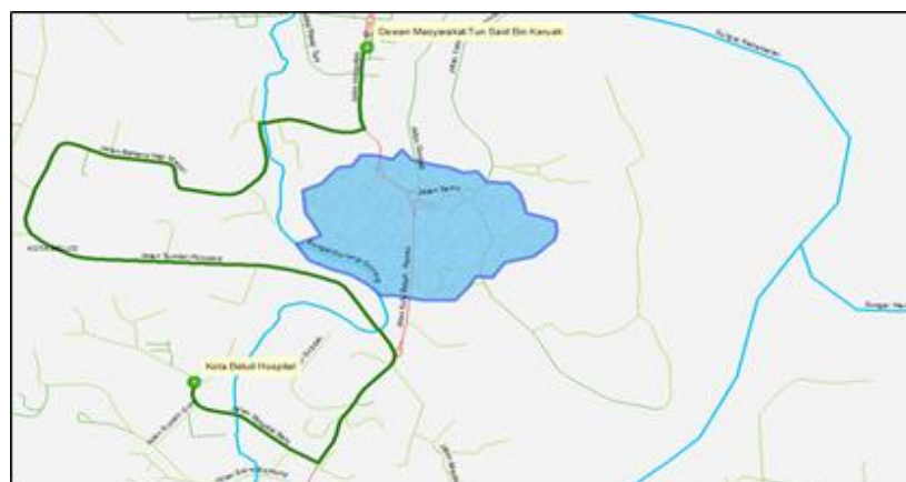
Figure 7. New/alternative route created using GIS network analyst, avoiding a flood event (design as polygon)
