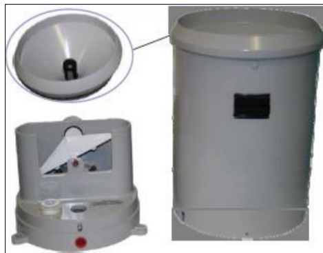
Figure 3. Tipping bucket used at the rain gauge station [16]
