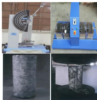
Figure 3. (a) Impact strength test, (b) slake durability test and (c) UCS sample at TD 2008
