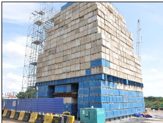
Figure 1. Reaction system by kentledge
