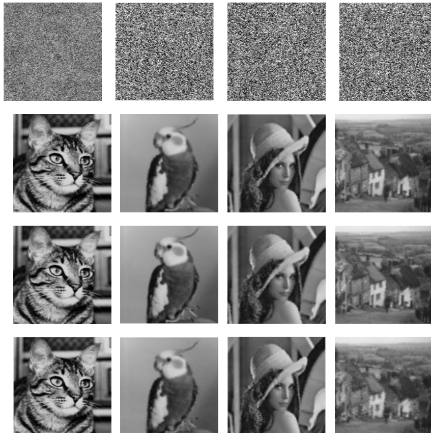
Fig. 3. Restoration of Cat, Bird, Lena and Goldhill. From top to bottom: noisy images with 90% salt-and-pepper noise, restorations obtained by the IRMIL, CG DESCENT, RMIL+ methods, respectively.
