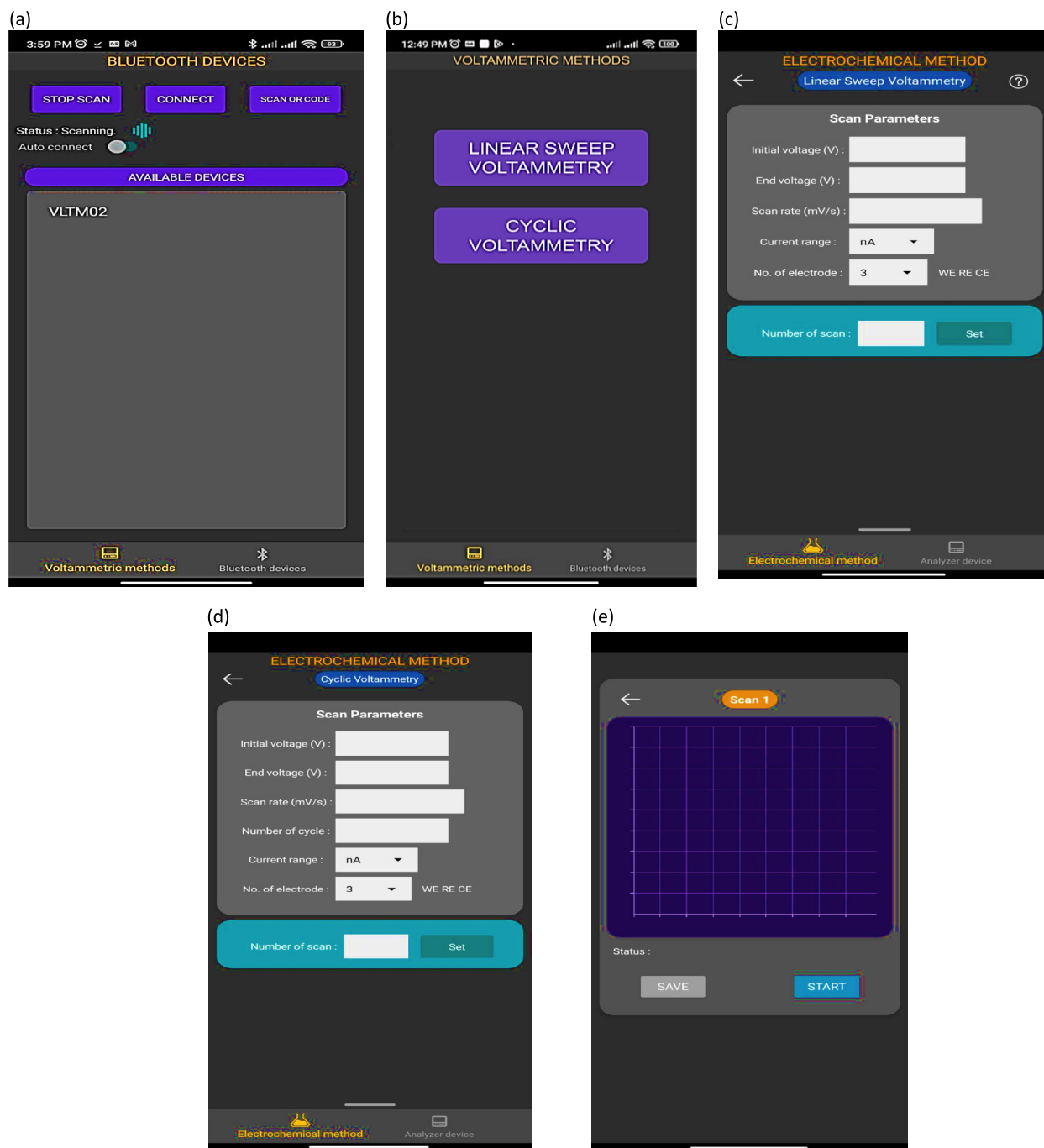
Fig. 18. Smartphone screen display designed features in 'Bluefruit Connect' app for (a) Bluetooth part of pairing with a potentiostat, (b) selection icon of mode measurements, (c) detail of specifications inputs for selection LSV mode (d) detail of specifications inputs for selection CV mode, and (e) graphical output and save data.
