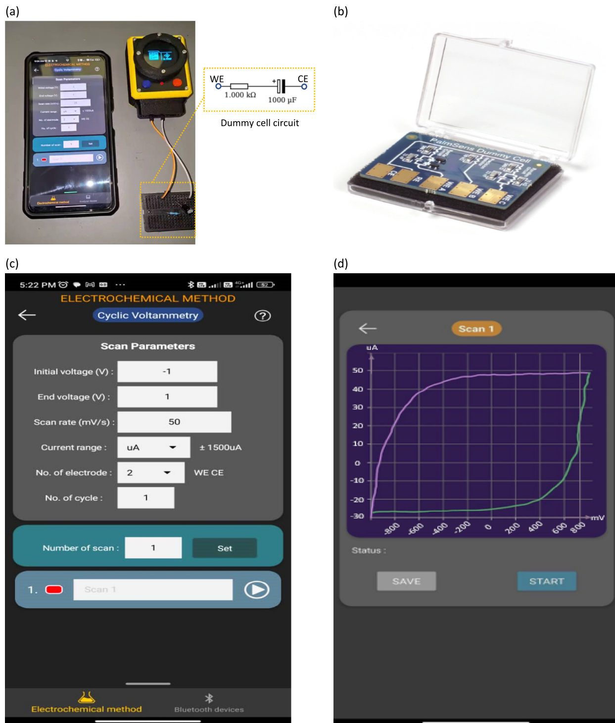
Fig. 21. Dummy Cell Testing. (a) Device set-up with connection of potentiostat and dummy cell. (b) Palmsens dummy cell. (c) Parameter values data in CV mode tab view. (d) CV measurement test using dummy cell.
