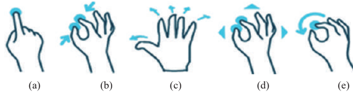
Figure 5 List of gesture inputs: (a) tap, (b) pinch, (c) release, (d) drag, (e) rotate.
