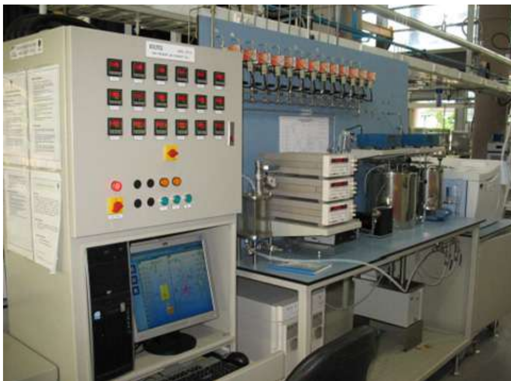
Figure 5. Experimental setup for CO 2 solubility study [55].
