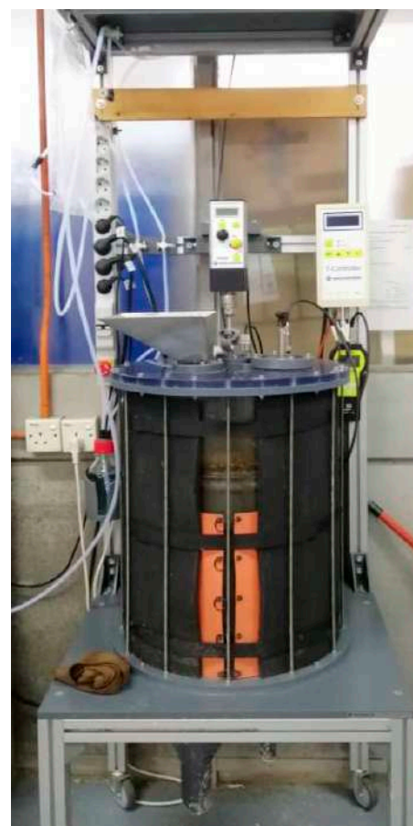
Figure 2. Schematic diagram and photo of Umwelteleistungen biogas test plant standard (BTP2). “1” refers to gas bag, “2” refers gas outlet valve, “3” refers to substrate inlet, “4” is meter, “5” is mixer blade, “6” is pH meter, “7” thermometer for substrate, “8” thermometer for gas, “9” large substrate outlet, and “10” small substrate outlet.
