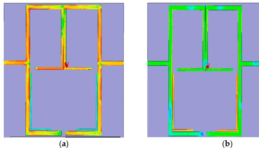
**Figure 15.** Nature of the current distribution of the triband filter (a) surface current density due to the frequency ratio K. (b) surface current density due to L-shaped resonator at 4.23 GHz.
