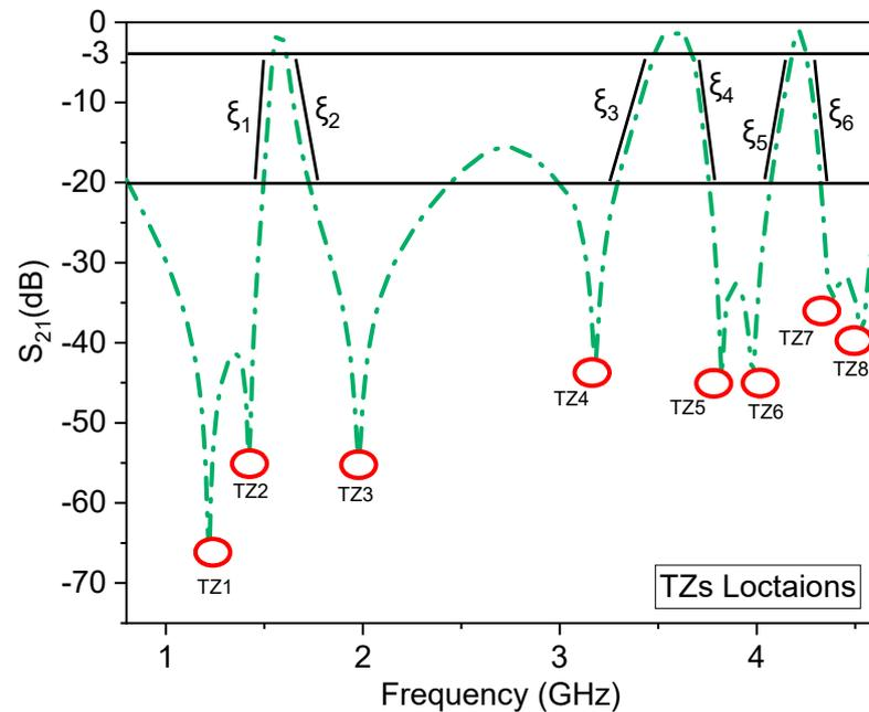
**Figure 9.** Location of T.Z.s at different frequencies with sharpness factor.
