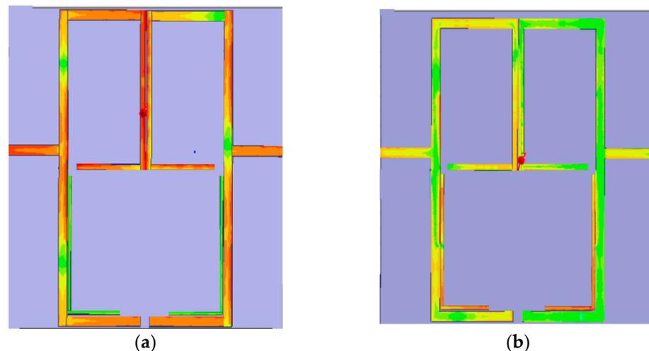
**Figure 16.** The magnitude of the electric field intensity (a) E due to the frequency ratio K. (b) E due to the L-shaped resonator at 4.23 GHz.
