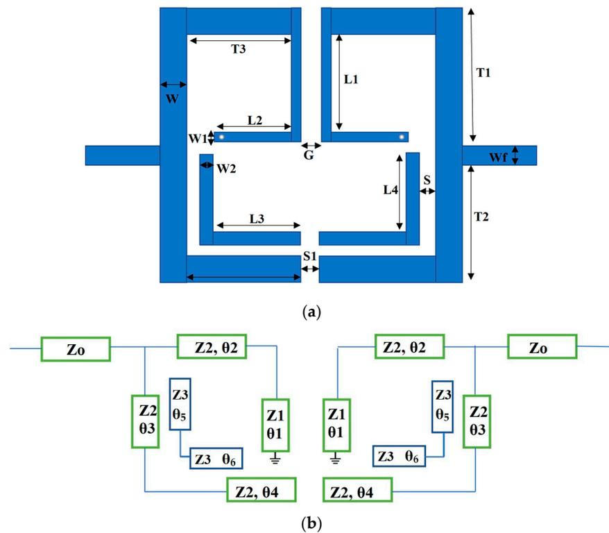
**Figure 3.** (a) Proposed triband geometry. (b) Equivalent circuit model.
