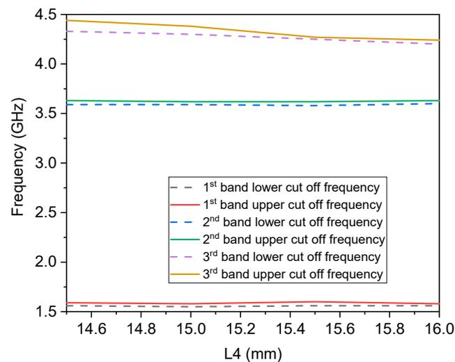
Figure 8. Variation in third pass band w.r.t stub length  $L_4$ .
