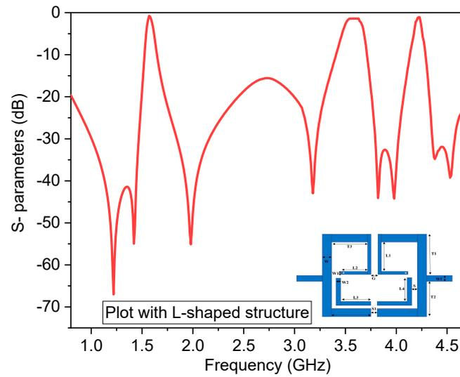
Figure 6. Realization of the third passband by embedded L-shaped resonator.
