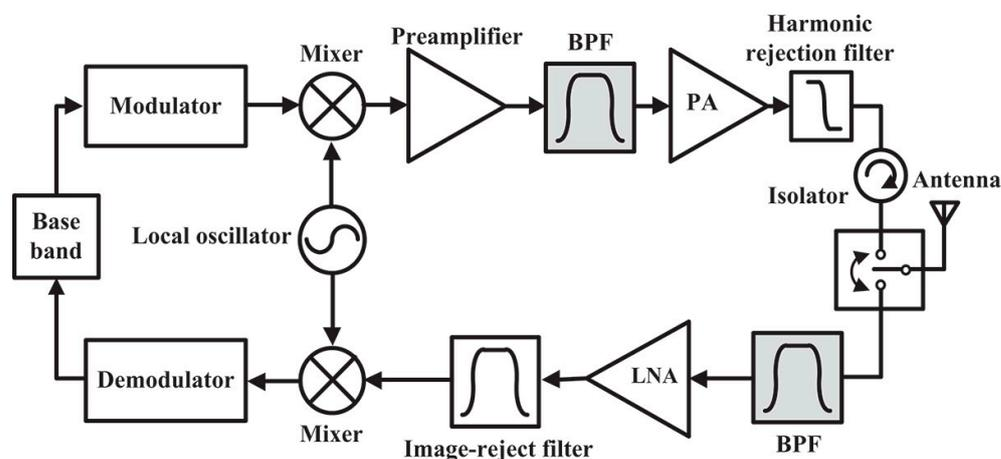
Figure 1. Placement of bandpass filter in communication systems [6].
