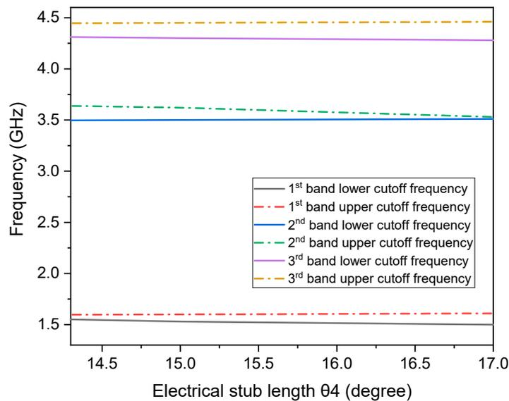
**Figure 5.** Variations in cut-off frequencies w.r.t electrical length  $\theta_4$ .
