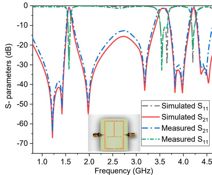
Figure 17. Simulated and measured  $S_{11}$  and  $S_{21}$  plots of the proposed geometry.
