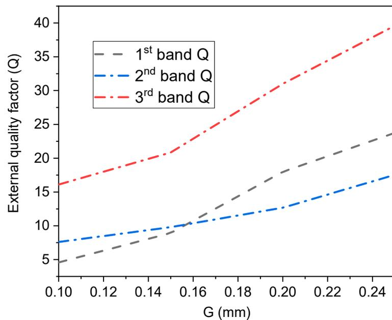
Figure 11. Effect of G parameter external quality factor on three passbands.
