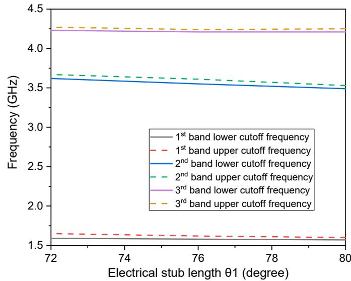
**Figure 4.** Variations in cut-off frequencies w.r.t electrical length  $\theta_1$ .
