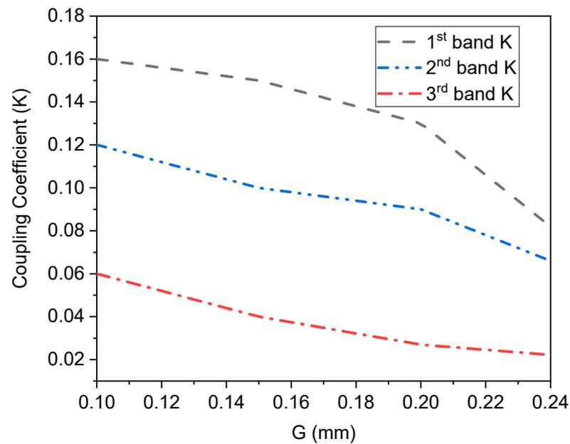
Figure 10. Effect of G parameter coupling coefficient on three passbands.
