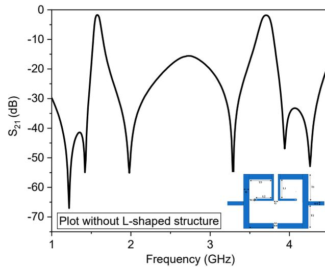
Figure 7. Response of filter without L-shaped structure.
