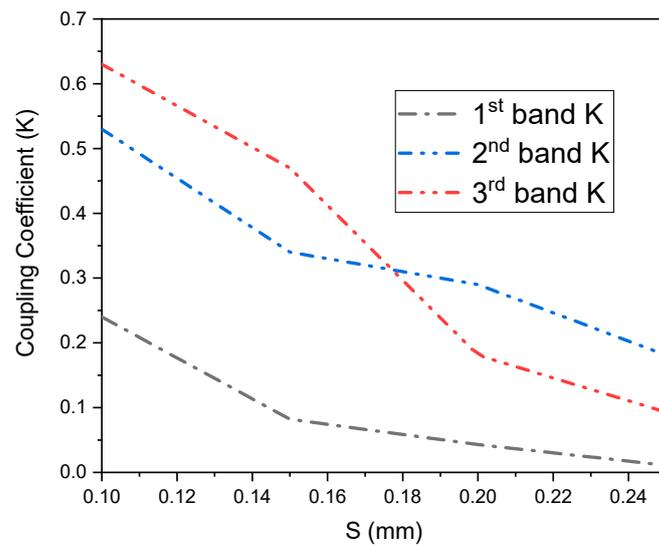
Figure 12. Effect of S parameter coupling coefficient on three passbands.
