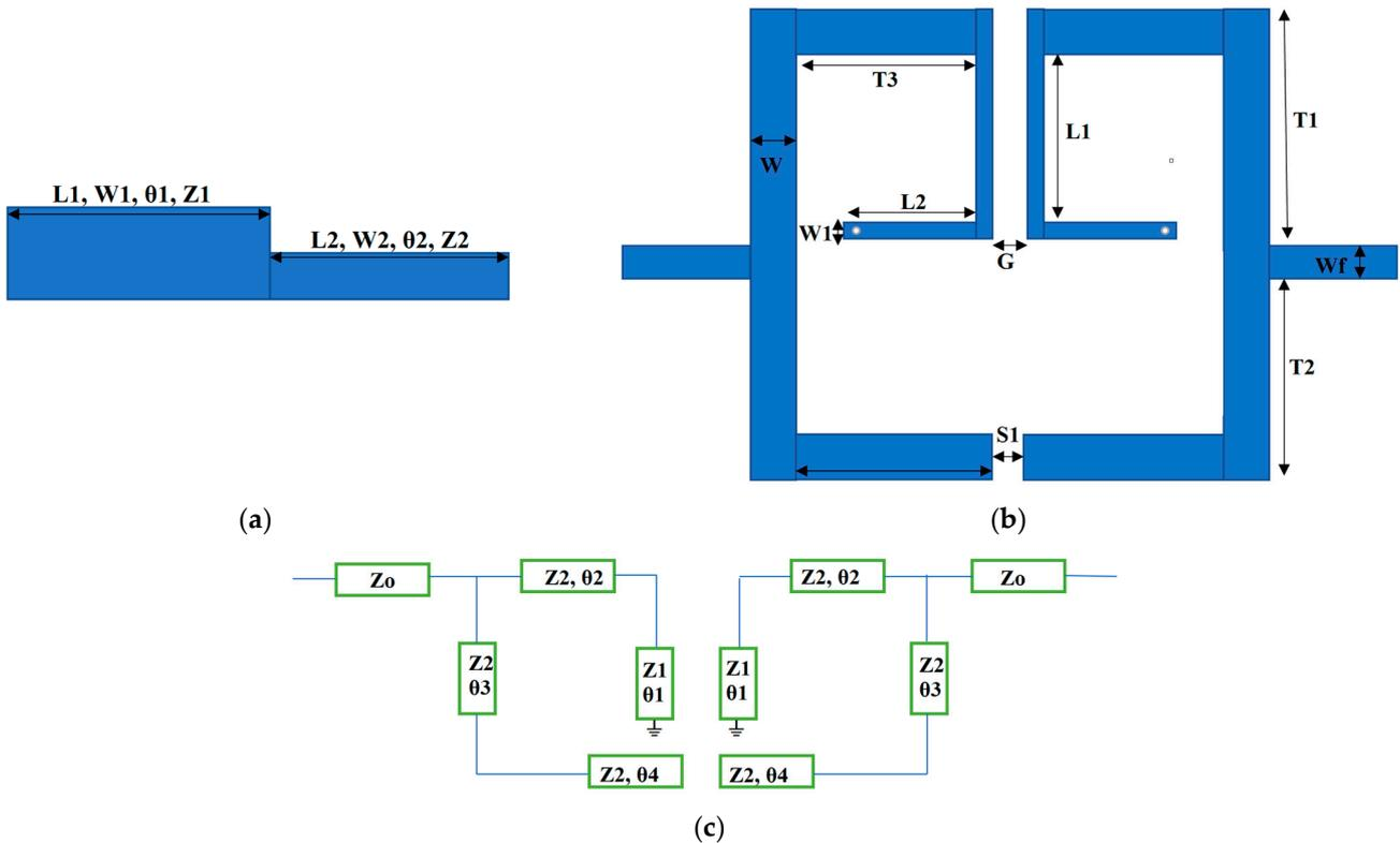
**Figure 2.** Configuration of resonators (a) Stepped impedance resonator (b) dual band filter topology (c) Equivalent structure of (b).
