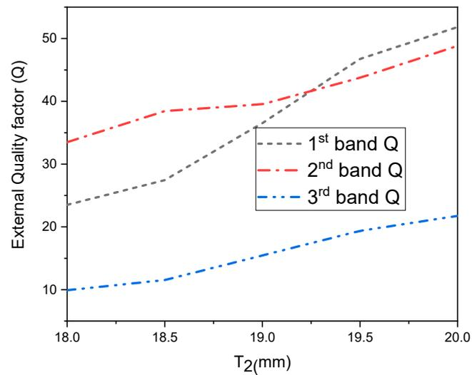
Figure 13. Effect of T<sub>2</sub> parameter external quality factor on three passbands.
