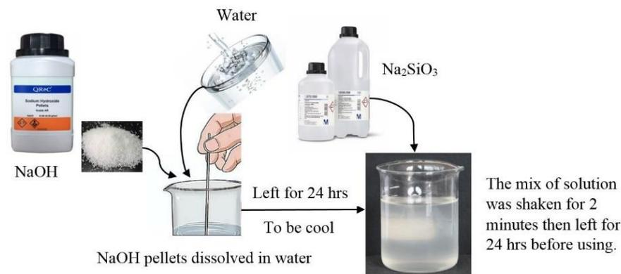
**Figure 4.** Preparation process of alkali activator solution Sodium hydroxide and sodium silicate bottles supplied by QREC [42].
