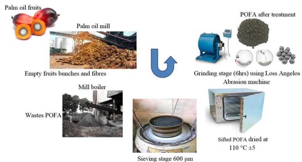
**Figure 1.** POFA treatment and processing, including collection, sieving, drying, and grinding [40,41].
