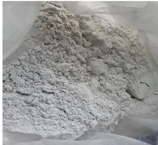
**Figure 2.** The utilized ground blast furnace slag (GBFS).
