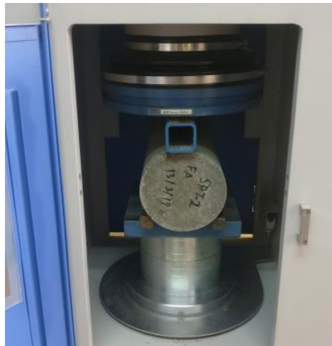
Figure A24 Experimental splitting tensile test setting
