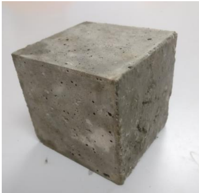
Figure A18 GPC specimens after heat cured and de-moulded
