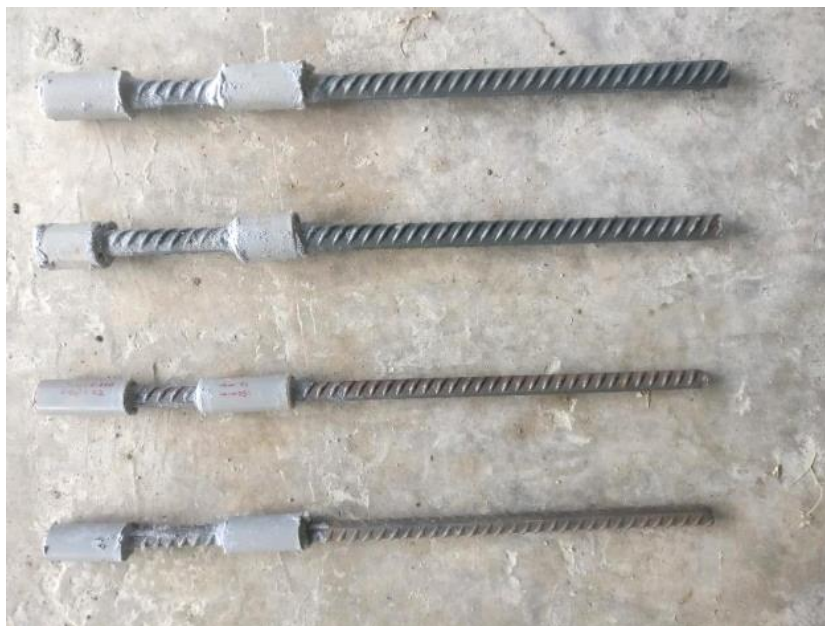
Figure A8 Bond breaker prepared for pull-out specimens
