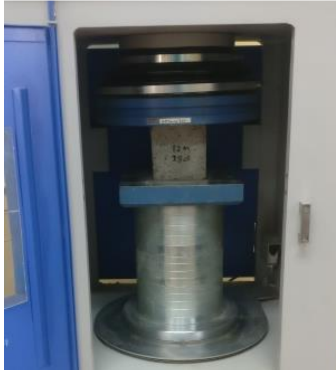
Figure A23 Experimental compressive strength test setting
