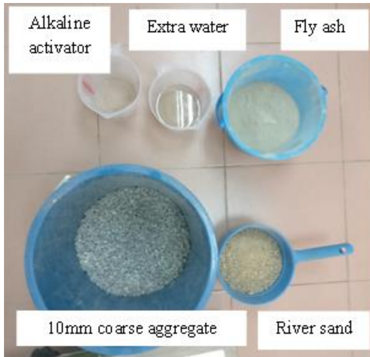
Figure A13 Materials to manufacture GPC specimens
