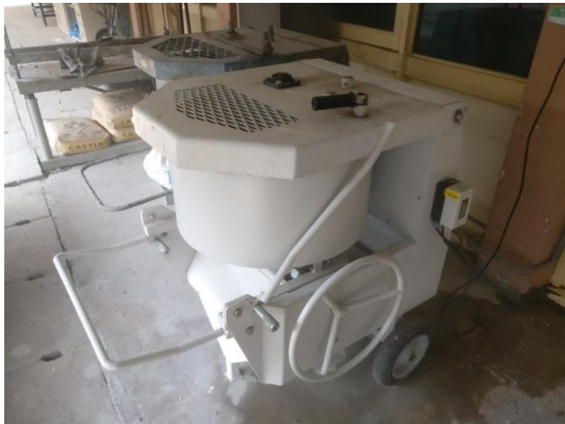
Figure A14 56-L capacity pan mixer
