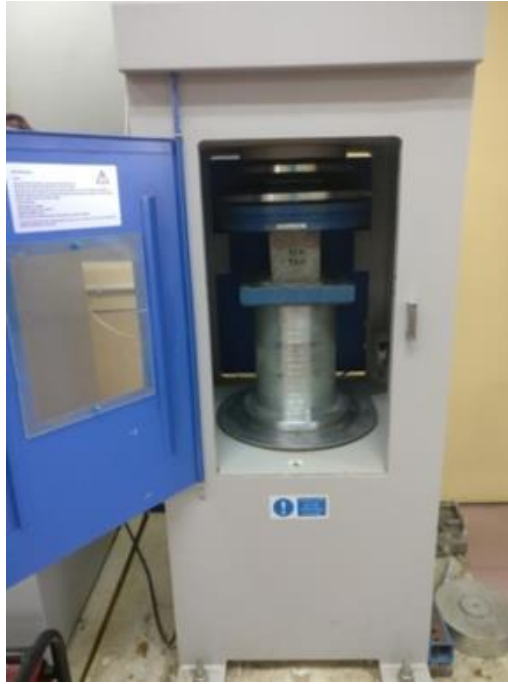
Figure A9 Universal Testing Machine for compressive and splitting tensile test
