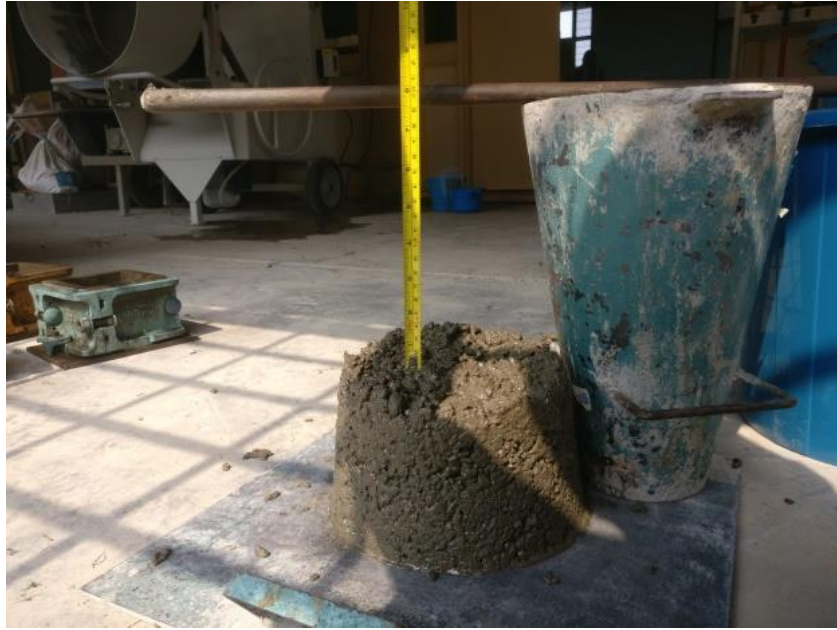
Figure A15 Workability test for GPC
