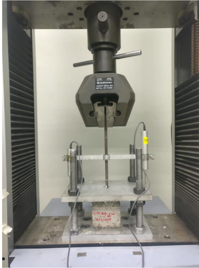
Figure A25 Experimental pull-out test setting
