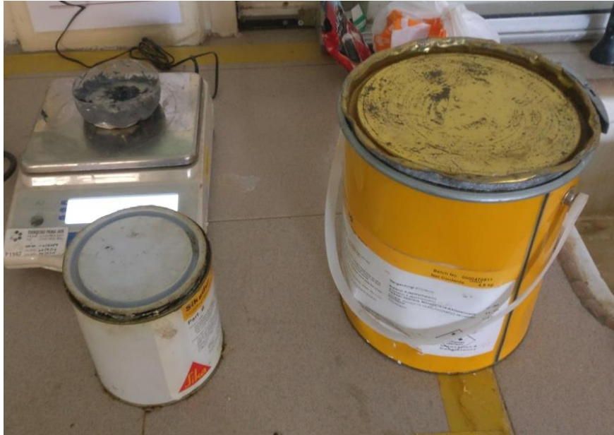
Figure A7 Sikadur-30 used to prepare the bond breaker
