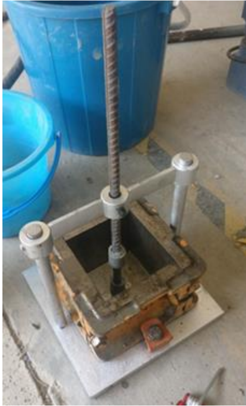
Figure A19 In-situ casting for 100 mm dimensional pull-out specimen
