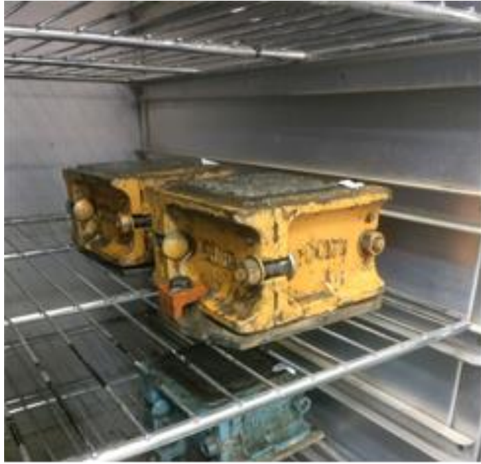
Figure A17 Dry oven curing for GPC
