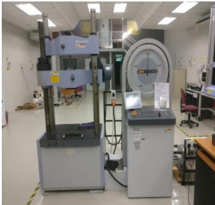
Figure A10 Universal Testing Machine for steel tensile test
