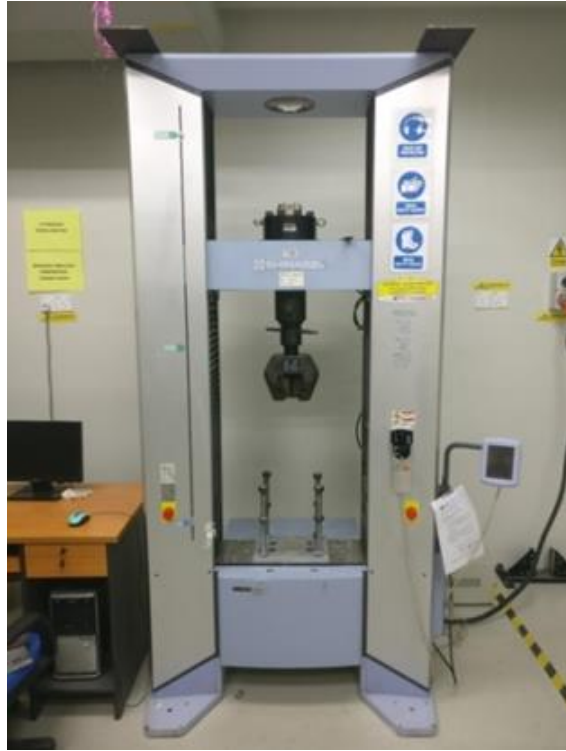
Figure A11 Universal Testing Machine for pull-out test
