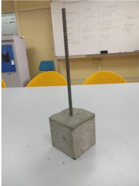
Figure A21 Pull-out specimen after de-moulding (a) 100 mm dimensional
