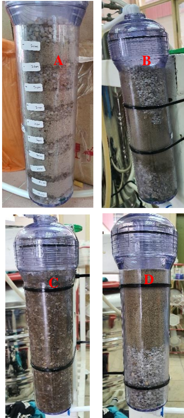
(A) Alternate arrangements of seaweed and fine silicone sand; (B) Seaweed layered between two-third of fine silicone sand portion; (C) Equally mixed seaweed and fine silicone sand; (D) Half seaweed and half fine silicone sand
