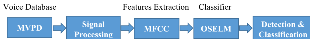
Fig. 2 Flowchart of voice pathology detection and classification using OSELM
