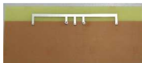
Figure 11. Fabricated two port shared radiator with shorting pins [72].
