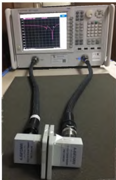
Figure 11. Experimental setup of array of the proposed model with vector network analyzed.
