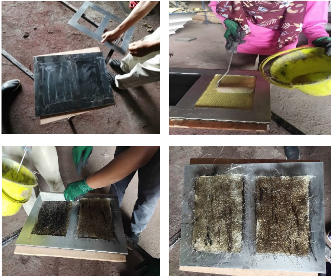
Fig. 2 – Fabrication process of natural fibres hybrid fibreglass/Kevlar composite materials.
