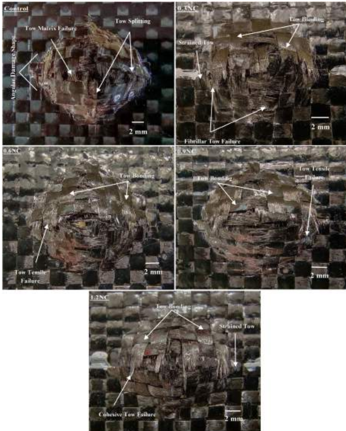
Fig. 12 – External damage of control and \text{NH}_2 -MWCNT reinforced carbon composites.
