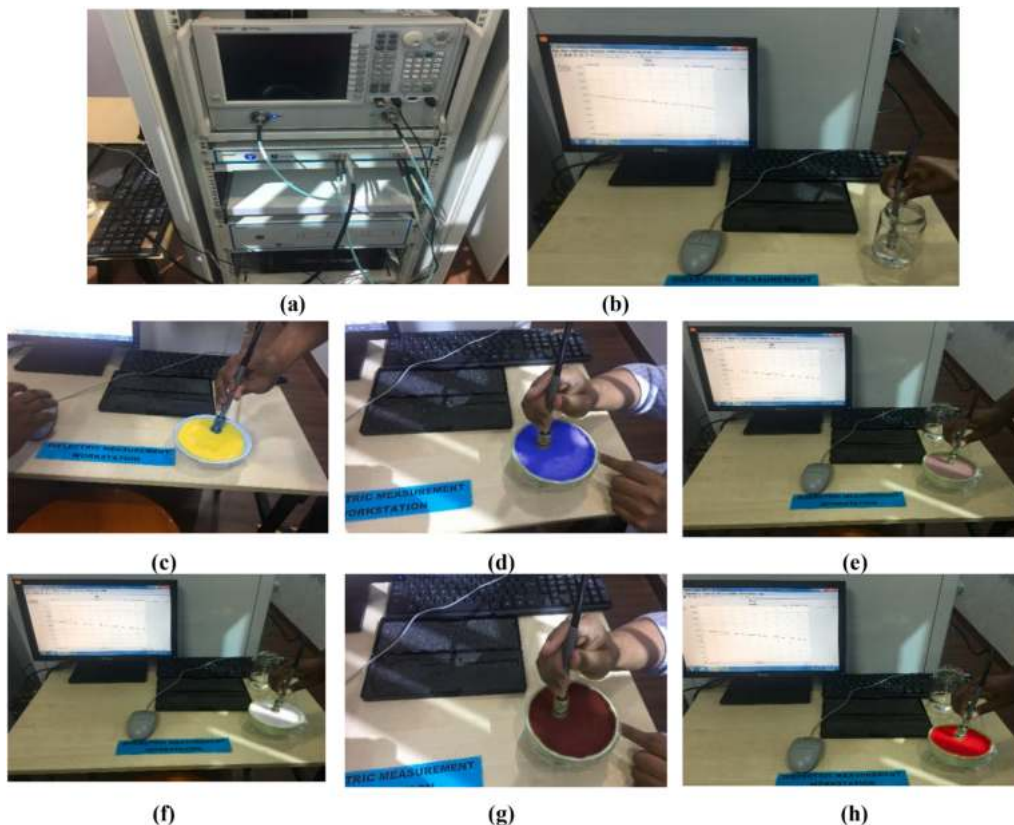
Fig. 7. The fabricated phantom measurement process and sample picture: (a) Experimental setup with PNA; (b) Sterile water calibration; (c) DUAR; (d) CSF; (e) Gray matter; (f) White matter; (g) Benign tumor; (h) Malignant tumor.
