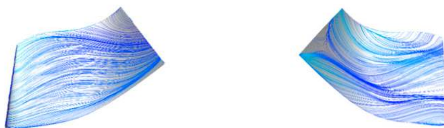
Figure 29. 30 K rpm flow topology of nozzleless turbine at off-design point.
