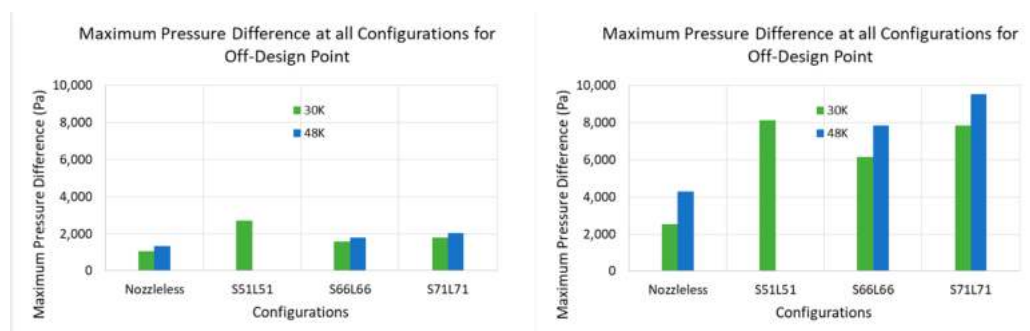
Figure 37. Maximum pressure differences between all configurations at both design and off-design conditions for both turbine speeds.
