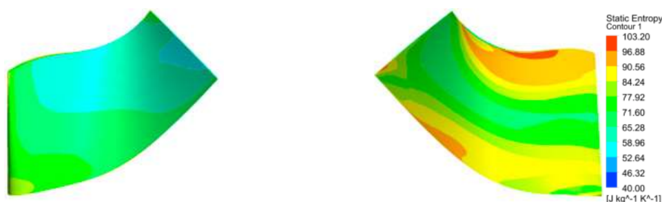
Figure 30. 30 K rpm entropy generation of nozzleless turbine at off-design point.
