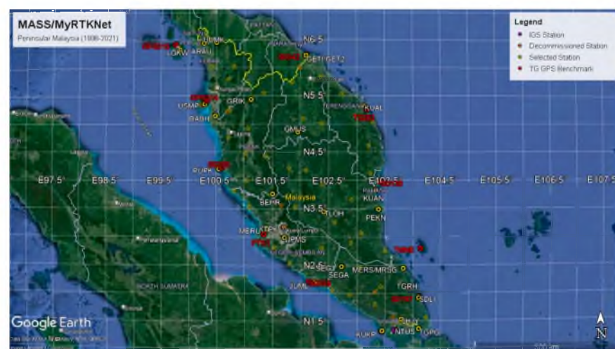
Figure 6. Location of 29 MASS/MyRTKNet stations at 20 locations (of which 12 are near the tide gauges) in Peninsular Malaysia. Shown also are the 11 tide-gauge benchmarks (in red, located below GETI/GET2). The tide-gauge benchmark at Johor Bahru unfortunately was lost during harbor reconstruction. Additionally, the other 60+ MyRTKNet stations currently operated by DSMM are shown (yellow open stars). The purple dot shows the NTUS station in Singapore which is part of the International GNSS Service (IGS) network. Yellow indicates still active and orange discontinued stations. Image made with Google Earth Pro.
