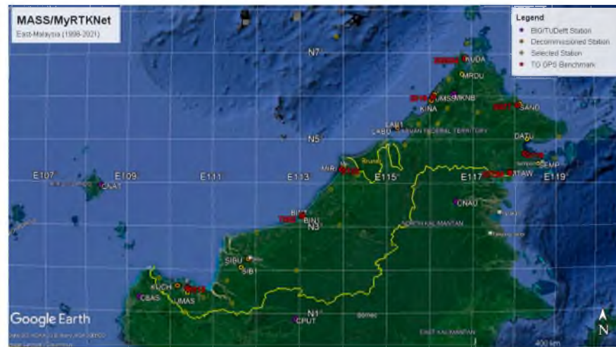
Figure 7. Location of 17 MASS/MyRTKNet and 1 GEODYSSSEA stations at 12 locations (of which 9 are near the tide gauges) in East Malaysia. Shown also are the 8 tide-gauge benchmarks (in red). Additionally, the 20+ other MyRTKNet stations (including 3 off-shore) currently operated by DSMM are shown (yellow open stars). The purple dots show the Indonesian InaCORS stations (CNAT, CBAS, CPUT, and CNAU) in the Indonesian part of Borneo (Kalimantan) as well as the TU Delft station MKNB on Mount Kinabalu in Sabah. Yellow indicates still active and orange discontinued stations. Image made with Google Earth Pro.
