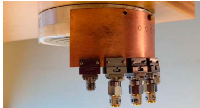
Figure 28. Patch antenna feeding the Luneburg lens.
