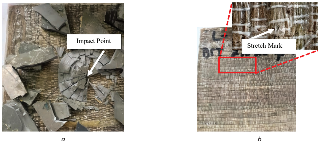
Fig. 15. Macrostructure of 3WC+10R: a – front side; b – rear side
