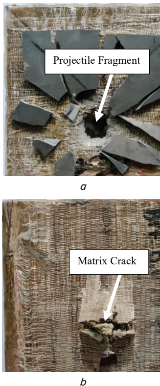
Fig. 10. Macrostructure of 1WC+10R: a – front side; b – rear side hard steel core
