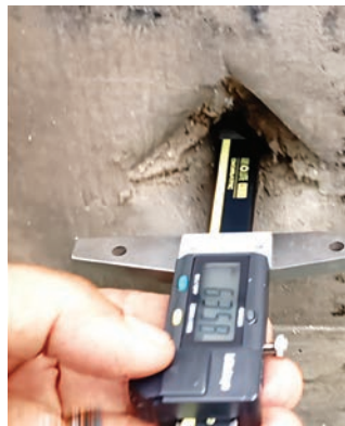
Fig. 7. Back face signature measurement illustration
