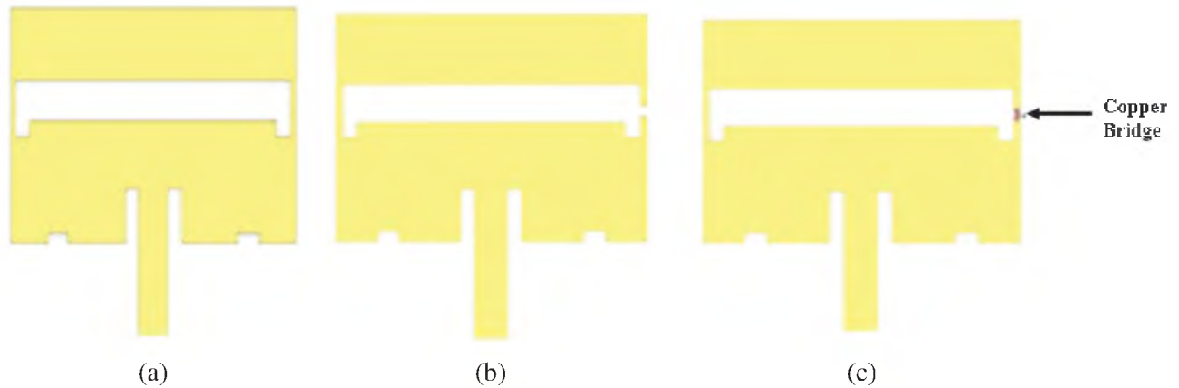
Figure 2. Proposed antenna at three design stages: (a) without a PIN diode, (b) without a copper bridge (OFF state), (c) with a copper bridge (ON state).
