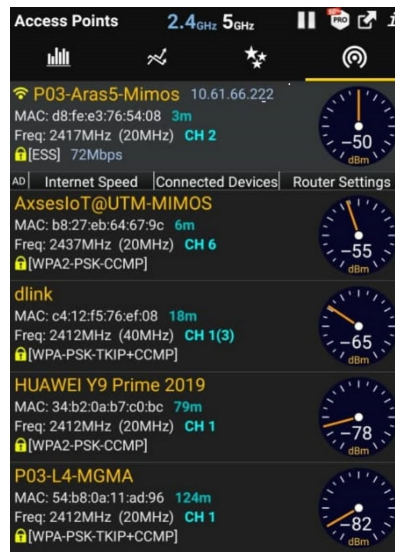
Figure 5. Screenshot of the Android application, WiFi Analyzer used for AP identification and labeling.
