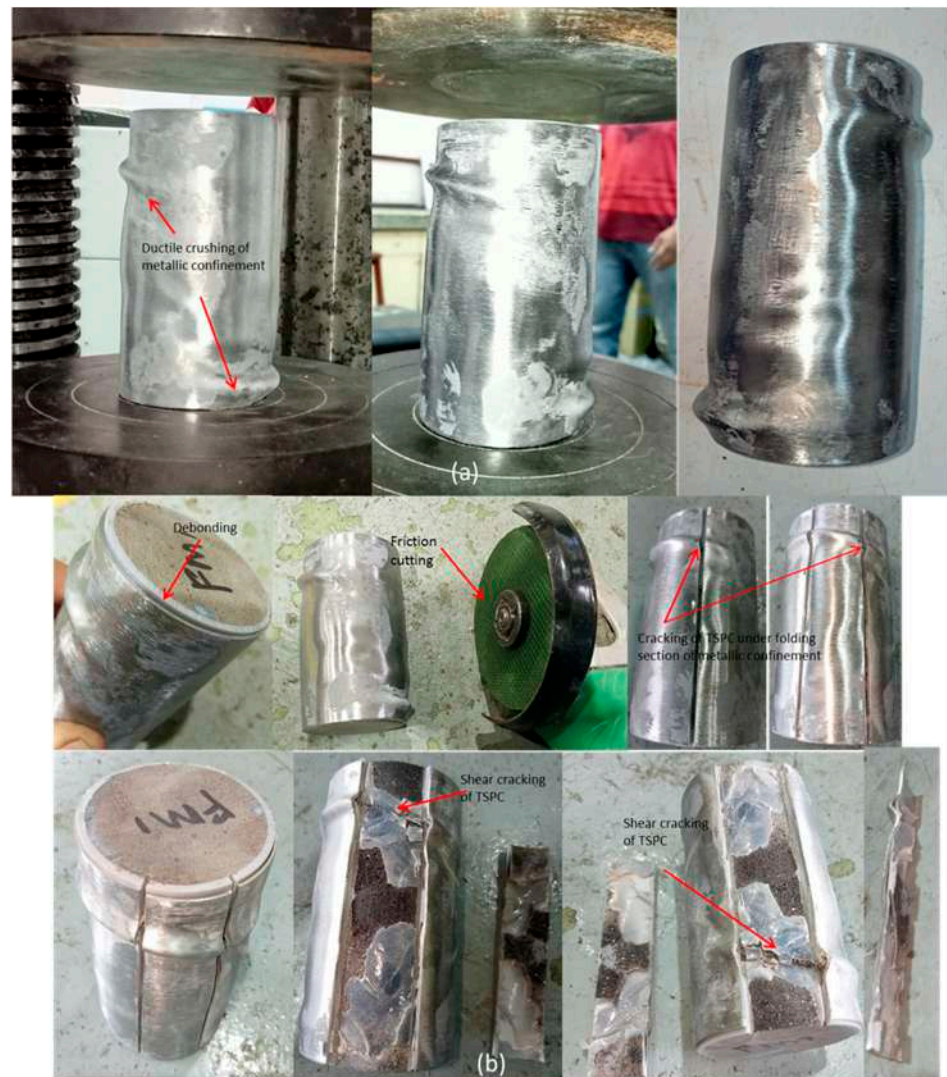
Figure 12. Failure modes of TSPC with fully metal tube confinement. (a) FM sample condition after mechanical testing. (b) The cut open of metal tube confinement for internal failure examination.
