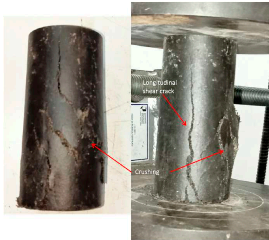
Figure 10. Failure modes of unconfined TSPC (UC).
