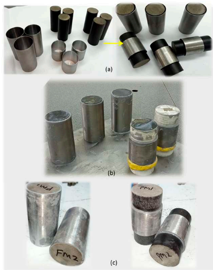
Figure 5. Specimen fabrication process. (a) Metal tube ready to confine the TSPC column. (b) Application of Sikadur 330 adhesive and curing of TSPC with metal tube confinement (binder thickness 0.5–1.0 mm). (c) Finished samples consist of TSPC with full and partial metal tube confinement specimens.
