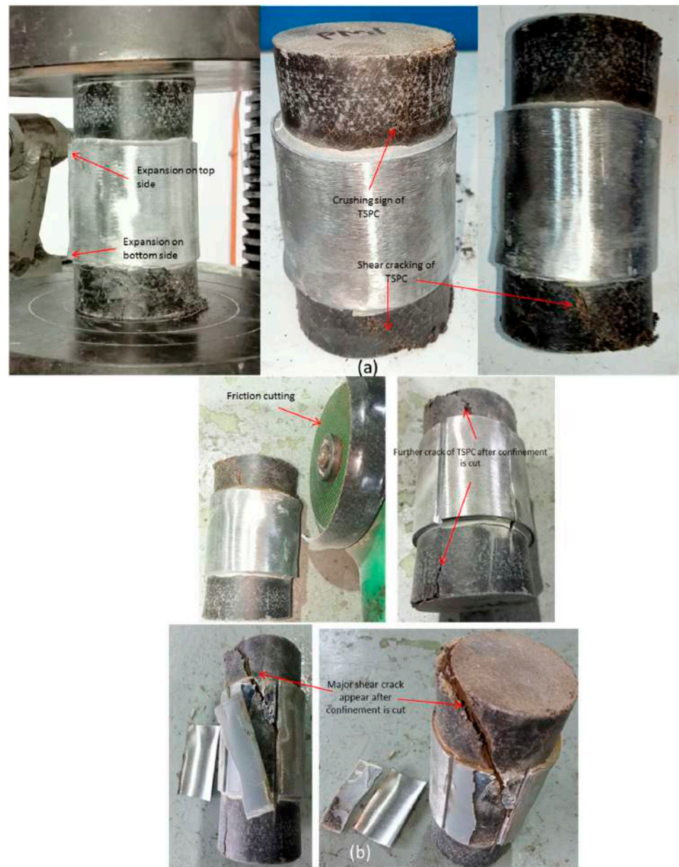
Figure 11. Failure modes of TSPC with partial metal tube confinement. (a) PM sample condition after mechanical testing. (b) PM sample with bottom side view and the cut open of confinement for failure examination.
