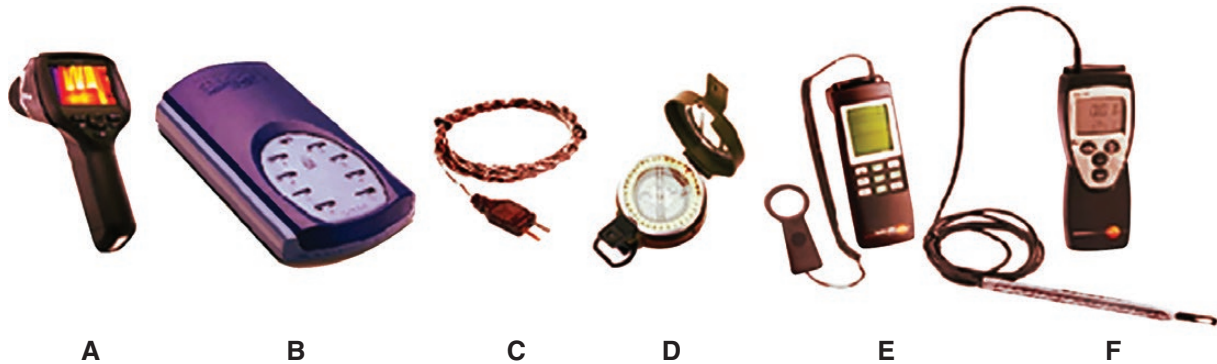
Fig. 5: Measurement devices used. (a) Infrared camera; (b) TC-08 data logger; (c) K-type thermocouples; (d) compass; (e) lux meter; and (f) hygro-thermal anemometer.
