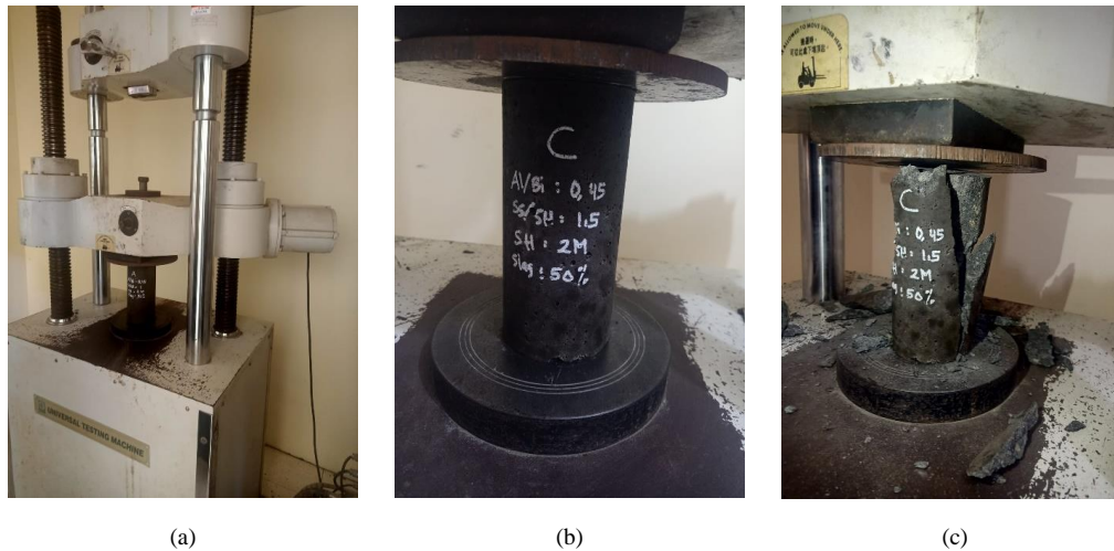
Figure 6. The compressive strength test: a) Universal Testing Machine, b) Specimen before testing, c) Specimen after testing
