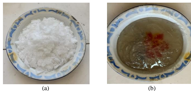
Figure 4. Alkaline activator (a) Sodium hydroxide, and (b) Sodium silicate
