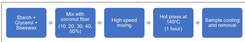
Figure 1. TPS/beeswax reinforced with coconut fiber
