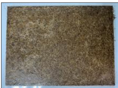
Figure 2. TPS/beeswax reinforced with coconut fiber
