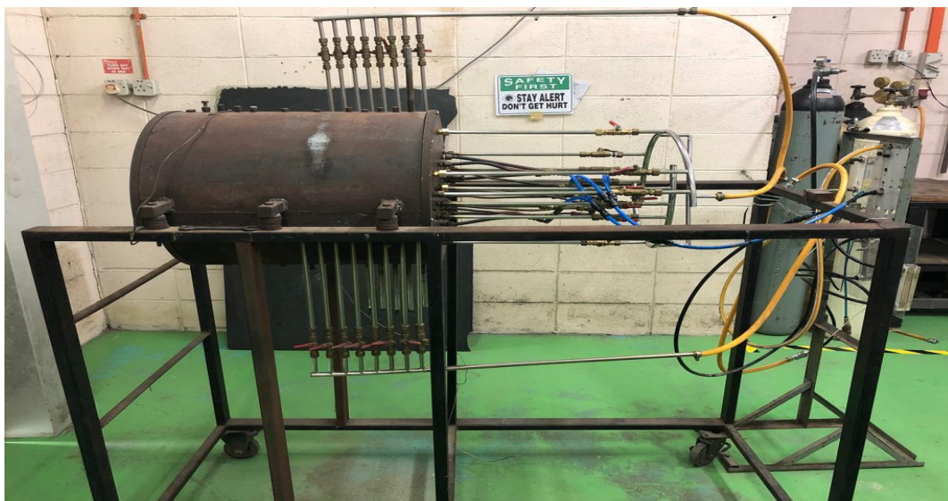
Fig. 2. Experimental setup of the asymmetric swirling combustor
