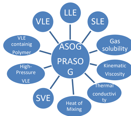
Fig. 2. Prediction of phase equilibria and transport properties using ASOG models
