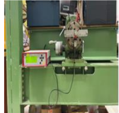
Fig. 15. Calibration set-up of the torque sensor
