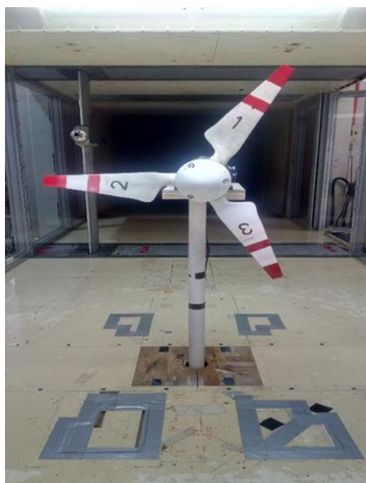
Fig. 5. Installation of the wind turbine model inside the section testing of the UTM-LST wind tunnel for testing
