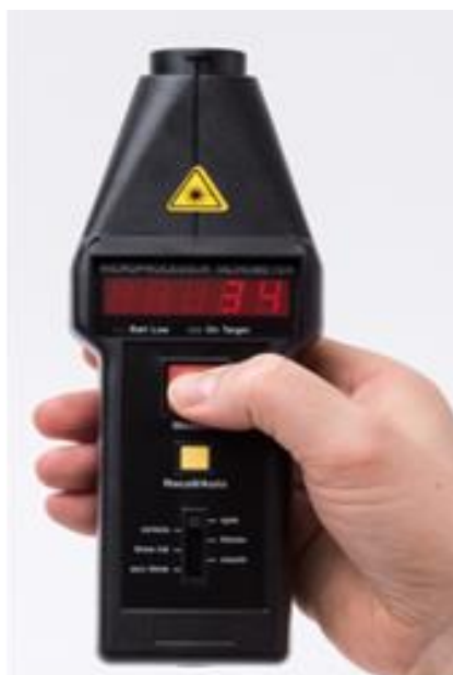
Fig. 17. Tachometer to measure the rotor blade rpm
