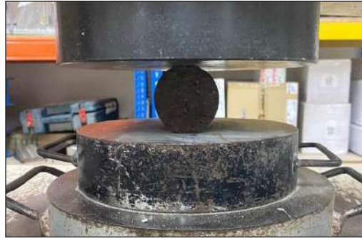
Figure 5. Lateral compression load of polymer concrete
