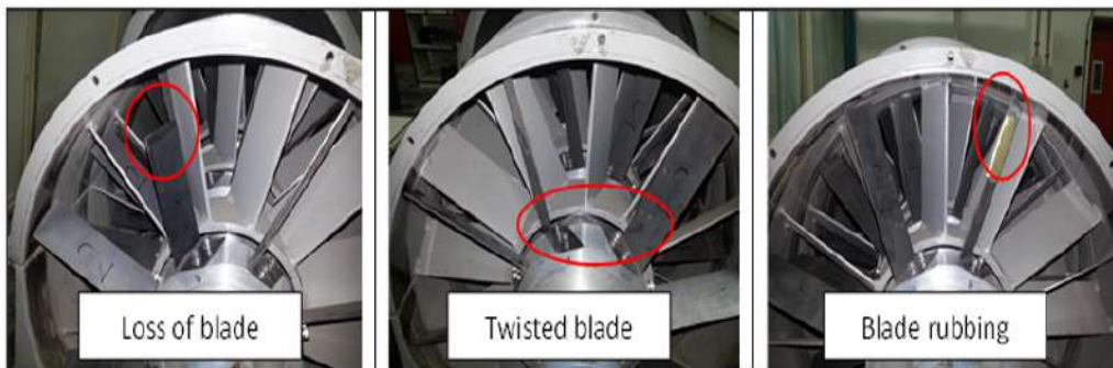
Figure 2. Type of blade faults
