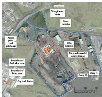
Fig. 2 Topside structures placement during onshore dismantling (Shell 2019)
