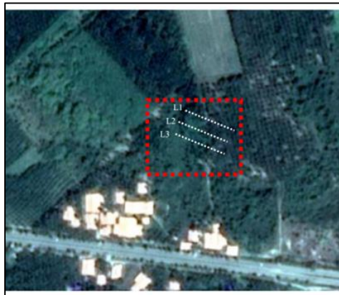
Fig. 3. The SPOT-7 satellite image captures the preliminary research region of Sungai Batu, Lembah Bujang. The red square box denotes the geophysical measuring area (electrical resistivity technique)
