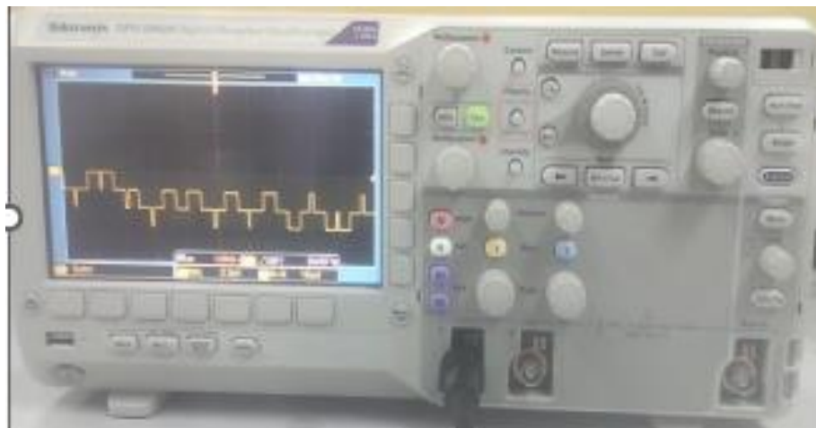
Fig. 1. The waveform captured from the oscilloscope. The V_{rms} was selected for the output voltage generated from the 360° lateral-sliding mode TEG
