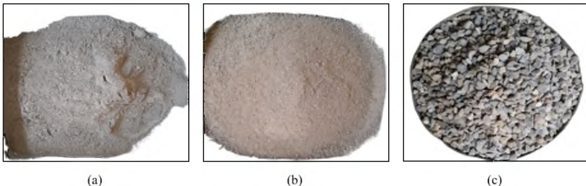
Figure 1: Basic ingredients of concrete (a) cement, (b) fine aggregates, (c) coarse aggregates.
