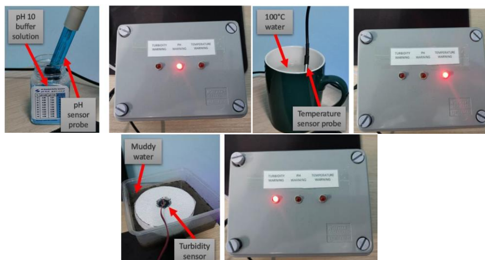
Fig. 13. The embedded warning system
